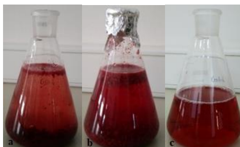
Figure 2- (a) Cornelian cherry extract prepared at 60 °C, (b) extract after 24 hours, (c) filtered extract
