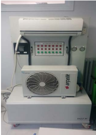
Fig. 4. Air conditioning training simulator system
