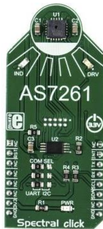
Figure 4. AS7261 XYZ Chromatic White Color Sensor
