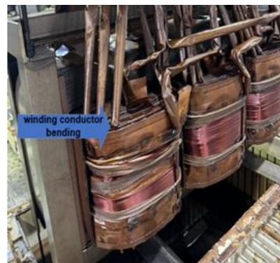
Figure 8. At maintenance facilities, mechanical and thermal deformations cause conductor burnout and bending failure.
