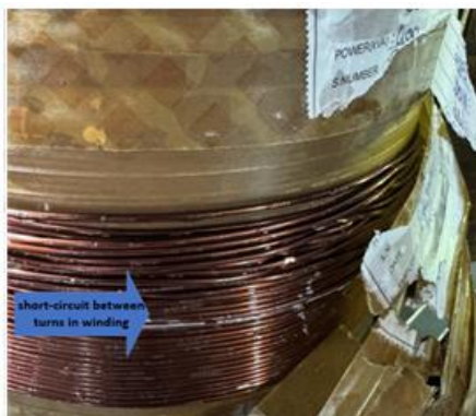
Figure 7. A short circuit between the windings
