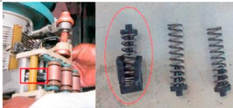
Figure 9. Example of drive mechanism failure in a voltage converter [5].
