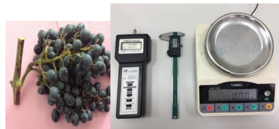
Figure 3. View of grape cluster, force gauge, micrometer and balance
