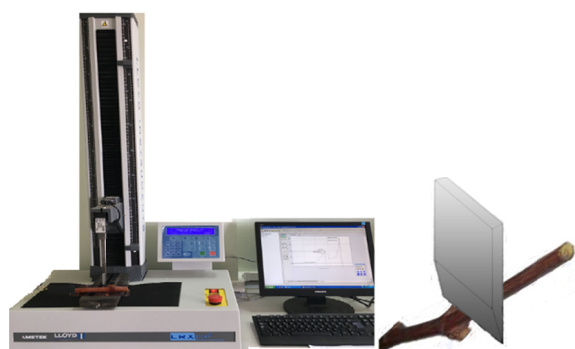
Figure 4. The Lloyd LRX Plus Materials Testing Machine and cutting blade
