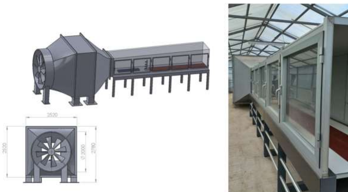
Figure 1. Wind tunnel test section and contraction cone views.
