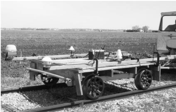
Figure 3. GPS receivers mounted on the rail car for testing (Taylor et al. 2004).
