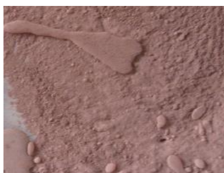
Figure 1. Water droplets escaping out of hydrophobe clay specimen.
