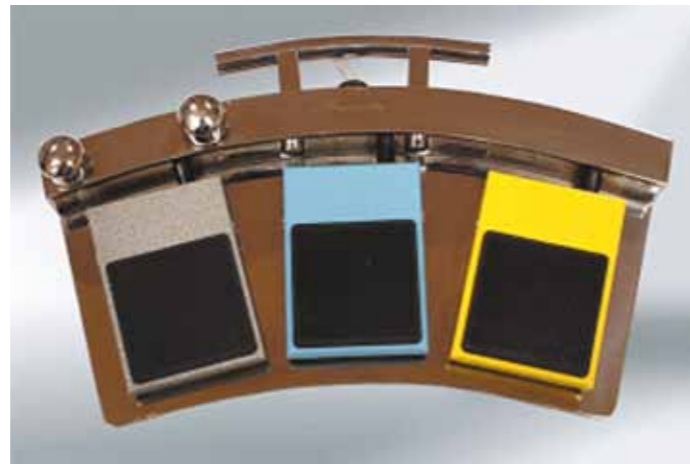
Figure 3: Special foot pedal to control the unit. Left pedal to aspirate only, the switches over the left pedal to increase or decrease the aspiration level, right pedal for ultrasonic lithotripsy and aspiration, middle pedal for pneumatic lithotripsy.
