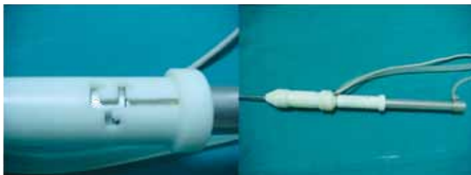
Figure 2: The ultrasound and Vibrolith combination; the Vibrolith probe is inserted into the hollow probe of the ultrasonic device.
