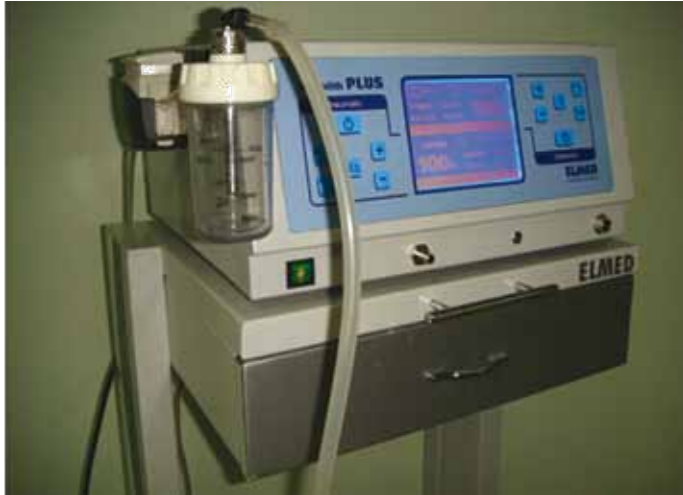
Figure 1: The control unit with the control elements for the ultrasonic lithotripter and the Vibrolith (pneumatic lithotripter).
