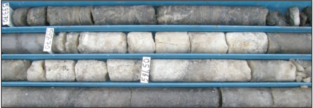
Figure 7- Bloedite-halite alternation cut in the drilling KEY-09/05 excavated in Konya-Ereğli-Yeniköy study (x: 4177106, y: 612493).
