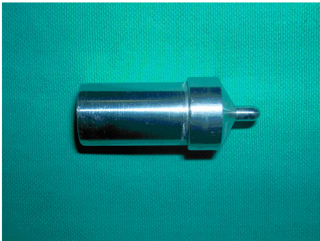
Figure 1. The probe with a 3 mm tip diameter for the application on rabbit lung.
