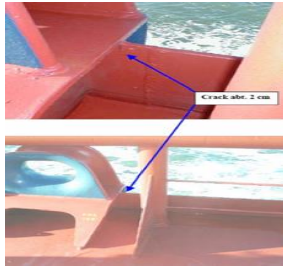
Figure 11. Cracks in gutter bar.
