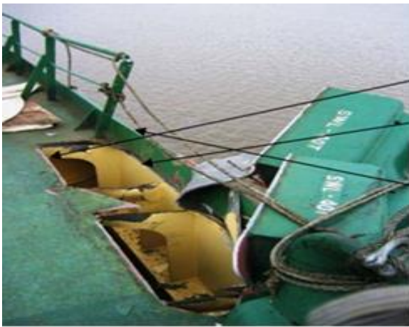
Figure 20. It shows 2 off 40 t SWL panama chocks torn off poop deck by tug.
