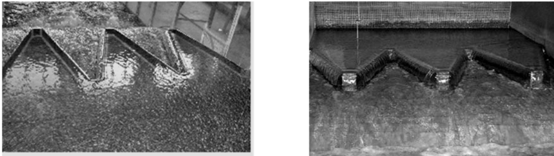
Figure 3. Experimental set-up for Trapezoidal labyrinth weirs
