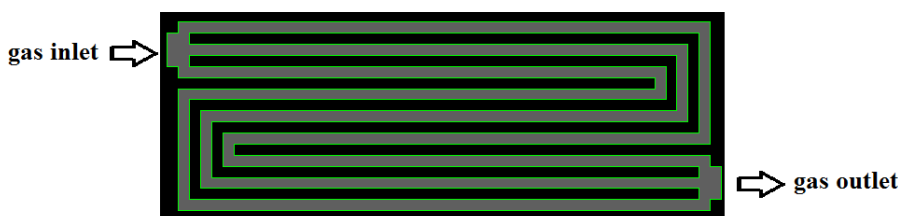
Figure 2. The bipolar plate flow channel pattern
