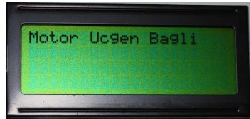
Figure 14. The state that the phase sequence is confirmed by the microcontroller and CRIM windings are delta connected.
