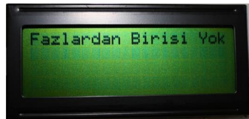
Figure 15. The state that the one of the phases is in fault.
