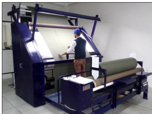
Figure 3. Traditional fabric defect inspection table.
