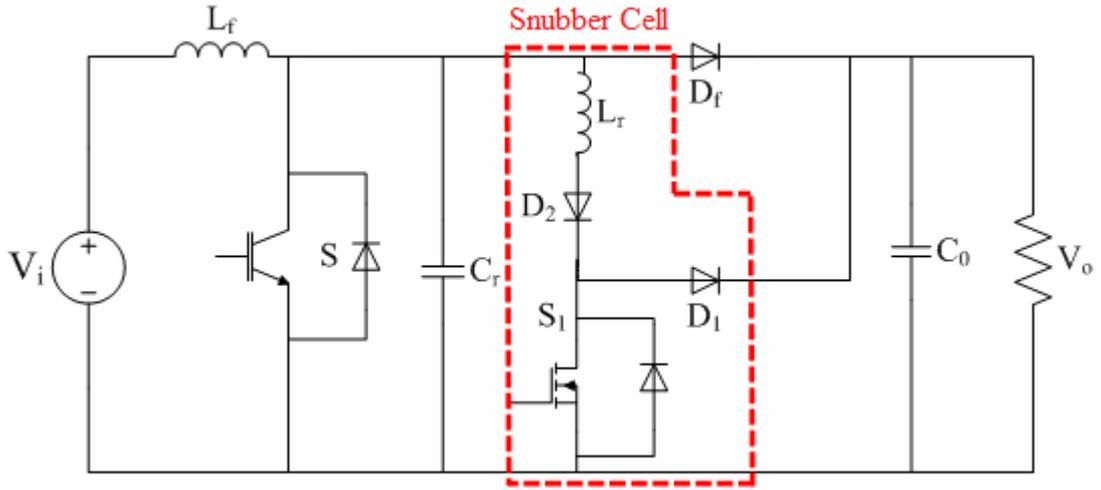
Figure 4. The basic ZVT converter circuit [5]
