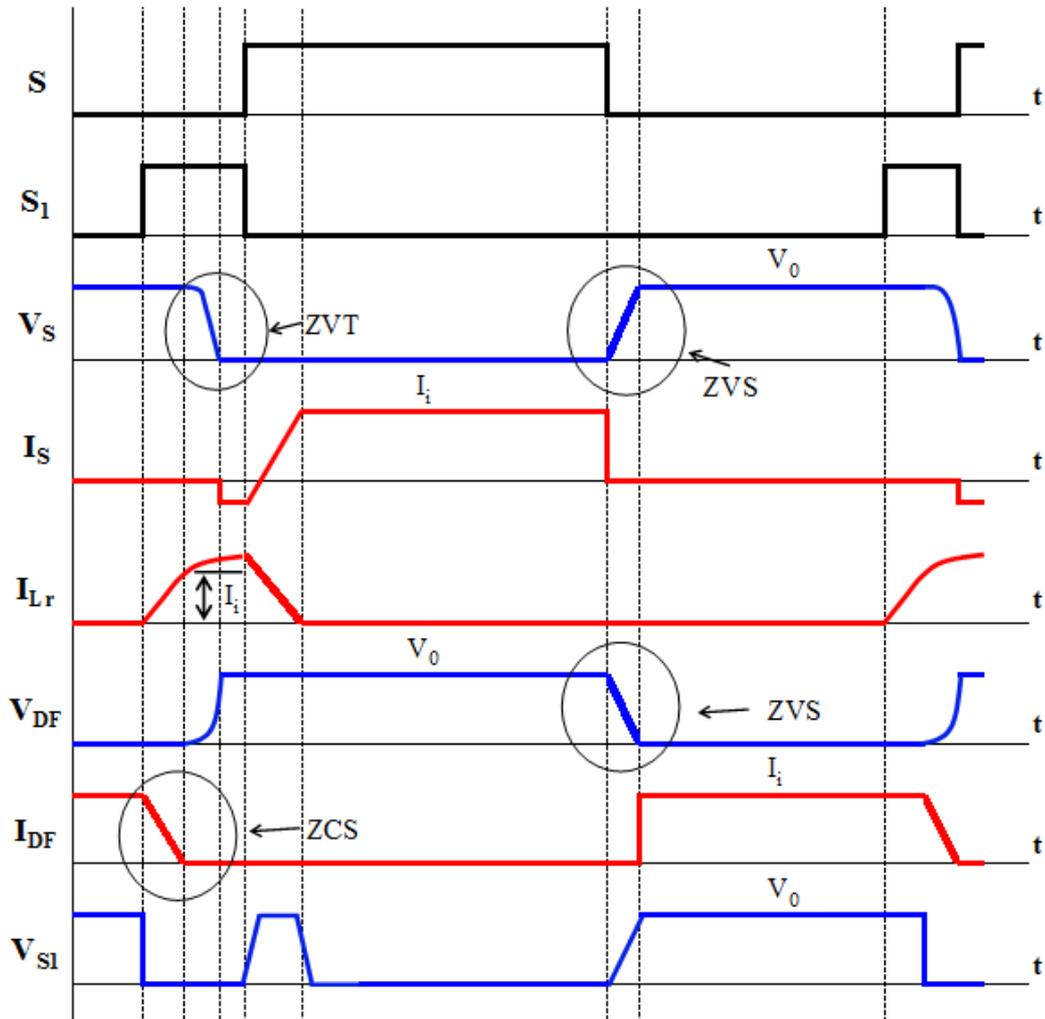
Figure 5. Switching signal of the main switch (S), switching signal of the auxiliary switch (S<sub>1</sub>), the main switch voltage (V<sub>S</sub>), the main switch current (I<sub>S</sub>) and L<sub>r</sub> inductance current (I<sub>Lr</sub>), the main diode voltage (V<sub>DF</sub>), the main diode current (I<sub>DF</sub>), the auxiliary switch voltage (V<sub>S1</sub>) [5]
