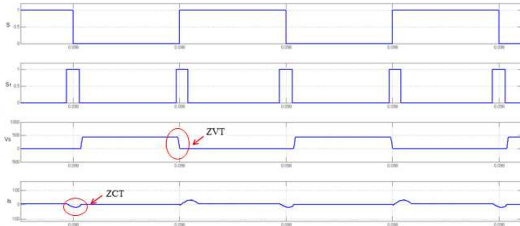
Figure 11. Switching signal of the main switch ( $S$ ), switching signal of the auxiliary switch ( $S_1$ ), the main switch voltage ( $V_S$ ) the main switch current ( $I_S$ )
