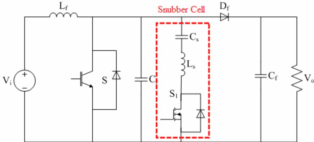
Figure 6. The ZVZCT DC-DC converter [7]
