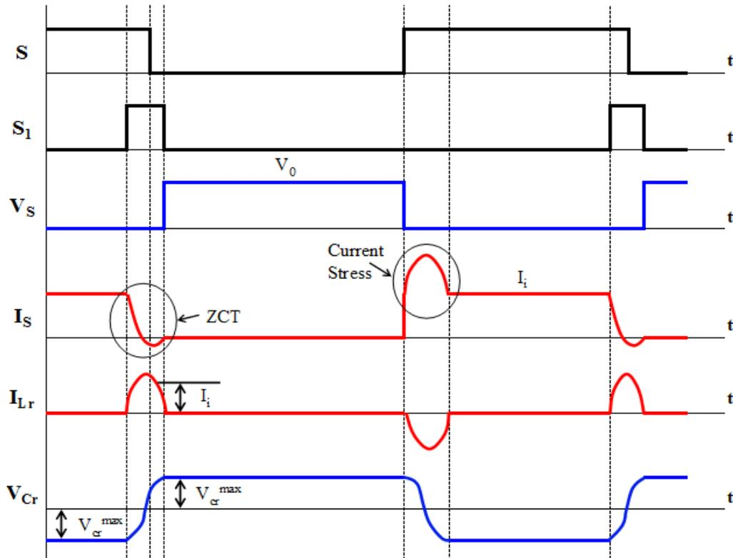
Figure 3. Switching signal of the main switch ( $S$ ), switching signal of the auxiliary switch ( $S_1$ ), the main switch voltage ( $V_s$ ), the main switch current ( $I_s$ ) and  $L_r$  inductance current ( $I_{Lr}$ ), the voltage of  $C_r$  ( $V_{Cr}$ ) [2].
