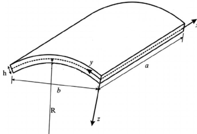
Figure 3. A cylindrical shell element
