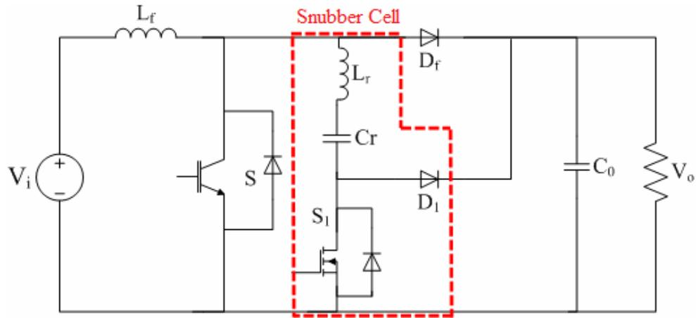
Figure 2. The basic ZCT converter circuit [2]
