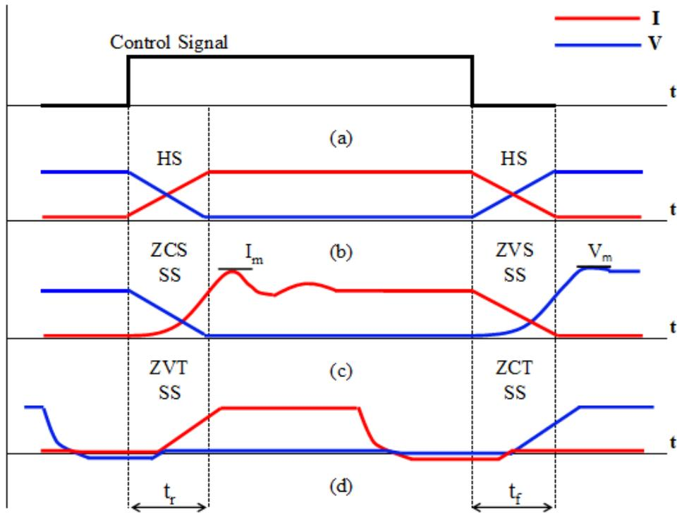
Figure 1. (a) Switching signal, (b) HS, (c) ZCS and ZVS, (d) ZCT and ZVT waveforms
