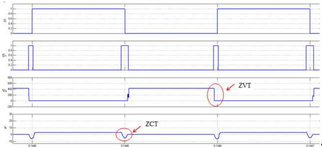
Figure 14. Switching signal of the main switch (S), switching signal of the auxiliary switch (S<sub>1</sub>), the main switch voltage (V<sub>S</sub>) the main switch current (I<sub>S</sub>)
