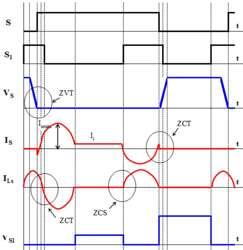
Figure 7. Switching signal of the main switch (S), switching signal of the auxiliary switch (S<sub>1</sub>), the main switch voltage (V<sub>S</sub>), the main switch current (I<sub>S</sub>) and L<sub>s</sub> inductance current (I<sub>Ls</sub>), the auxiliary switch voltage (V<sub>S1</sub>) [7]
