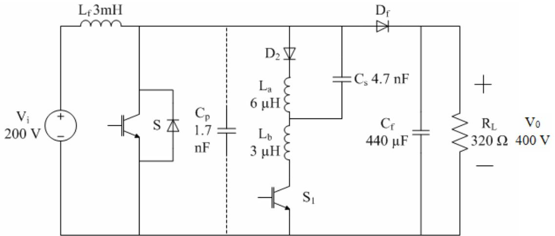
Figure 13. The model of ZVZCT Converter-II used in simulation [8]
