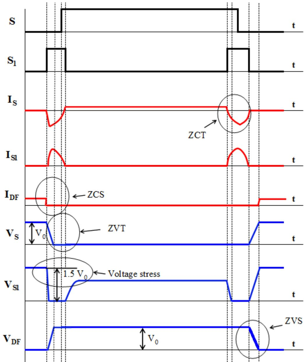
Figure 9. Waveforms of the semi-conductors in the converter [8]
