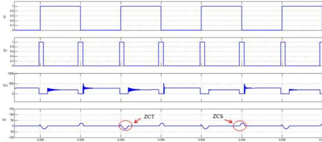
Figure 12. Switching signal of the main switch (S), switching signal of the auxiliary switch (S<sub>1</sub>), the auxiliary switch voltage (V<sub>S1</sub>) the auxiliary switch current (I<sub>S</sub>)
