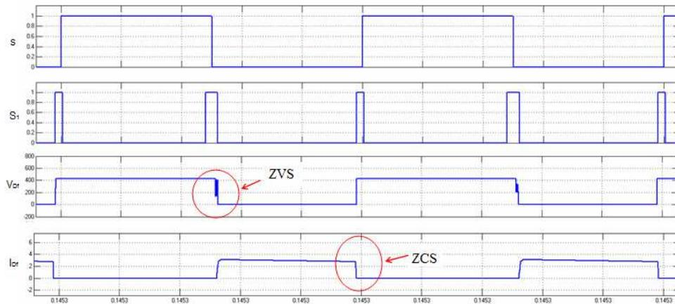
Figure 16. Switching signal of the main switch ( $S$ ), switching signal of the auxiliary switch ( $S_1$ ), the main diode voltage ( $V_{DF}$ ), the main diode current ( $I_{DF}$ )
