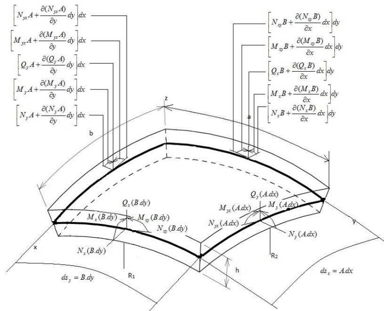
**Figure 2.** Forces and moments on shell element
