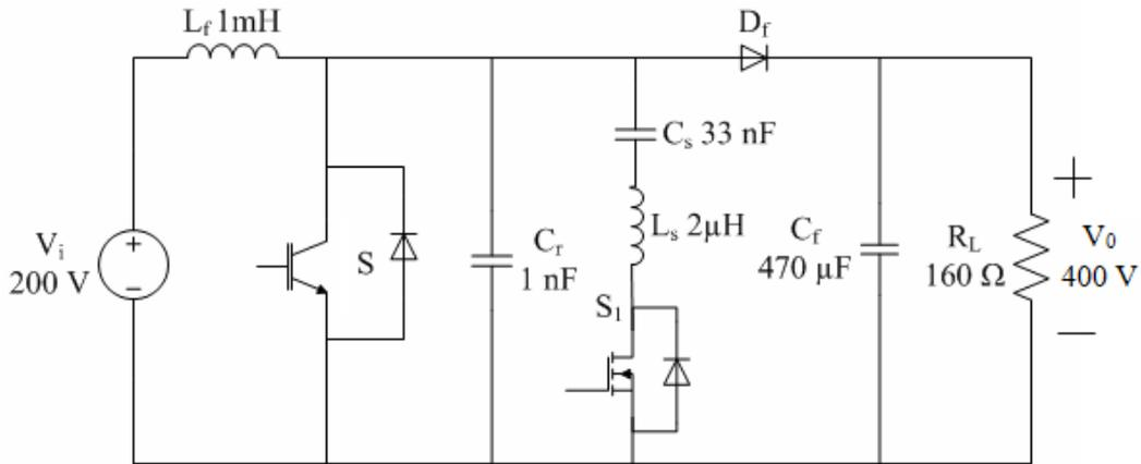
Figure 10. The model of ZVZCT Converter-I used in simulation [7]
