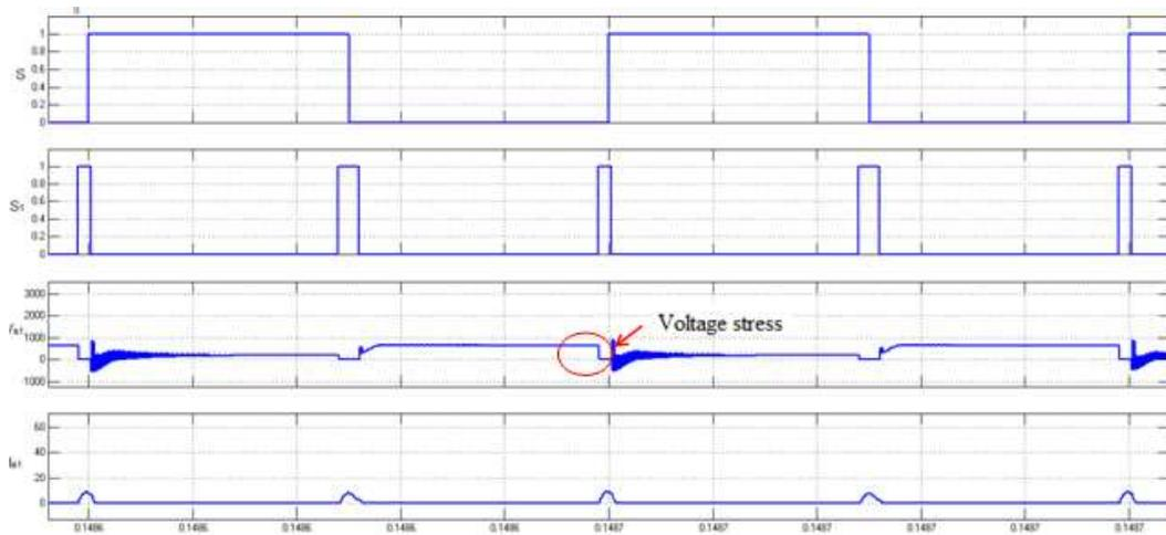
Figure 15. Switching signal of the main switch ( $S$ ), switching signal of the auxiliary switch ( $S_1$ ), the auxiliary switch voltage ( $V_{S1}$ ) the auxiliary switch current ( $I_S$ )
