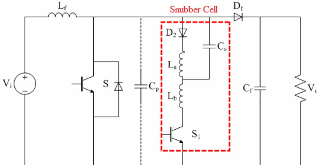
Figure 8. The ZVZCT DC-DC converter [8]
