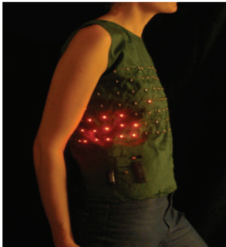
Figure 5. LED integrated clothing [12]
