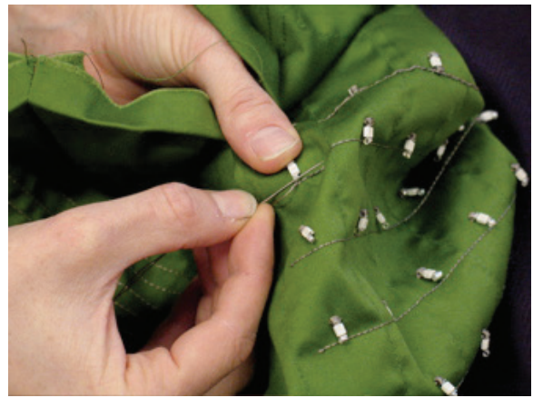
Figure 6. Conductive yarn with LEDs [14]
