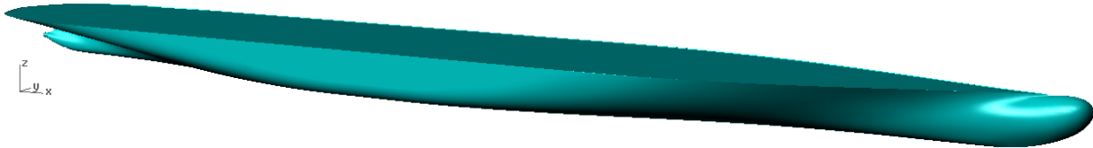
Figure 3. Perspective view of the underwater hull of the DTC model.
