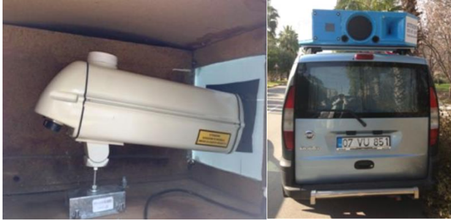
Fig. 4. ANPR setup placed on the vehicle
