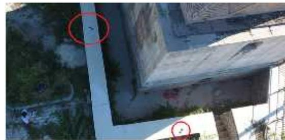
Figure 3. Establishing ground control points
