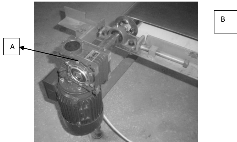
A- Electrical motor B-Band conveyor Figure 4. Picture of driver unit
