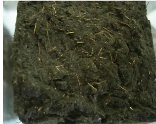
Figure 8. Pulled-out steel fibers
