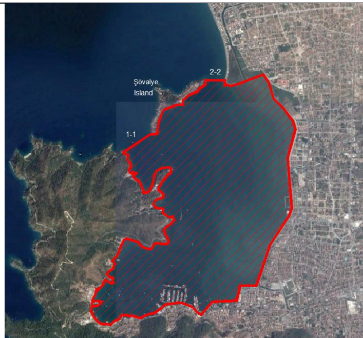
Figure 3. Computational cell utilized for the inner bay of Fethiye to simulate the mean water quality parameters. [20]
