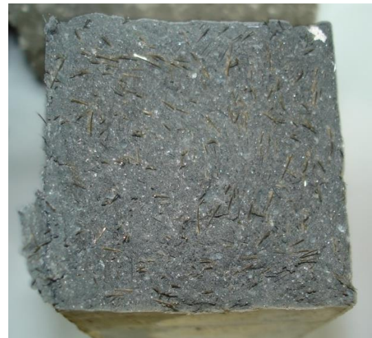
Figure 9. Ruptured waste erosion wires
