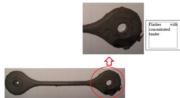
Figure 4. Specimen injected with pressure of 1100 bar, and flow rate of 30 cm 3 /s
