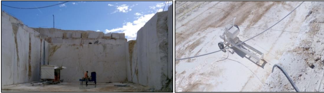
Şekil 13. Alt kesimde zincirli kollu kesicinin ve dikey kesimde elmas tel kesme kullanımı (The use of chain saw machine for underside cut and diamond wire cutting machine for the vertical cuts)
