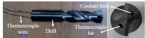
Fig. 2. The twist drilling tool and thermocouple inserted through the hole of internal coolant carbide drill[3, 4]
