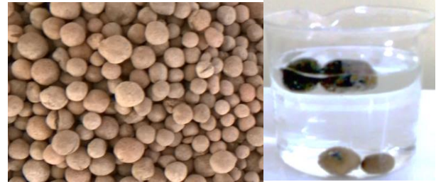
Şekil 4. Genleşmiş kil agregalar ve suda batma testi (Expanded clay aggregates and water penetration test)
