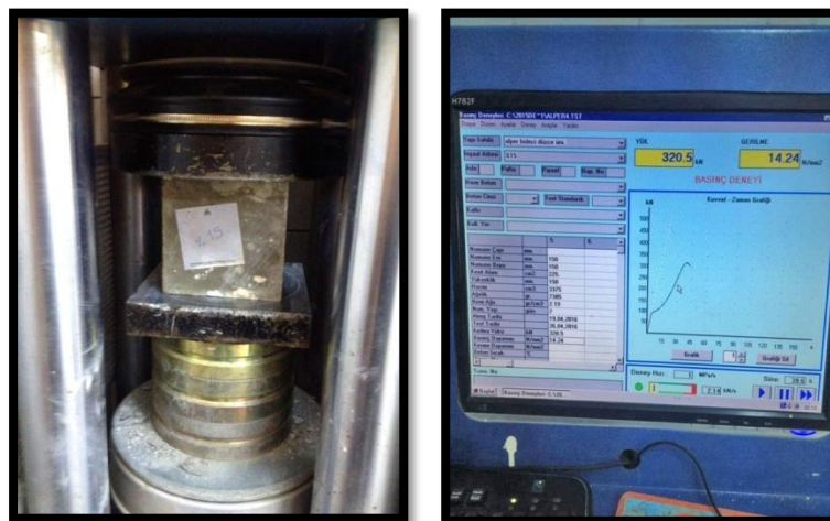
Fig. 4. Application of compressive strength test
