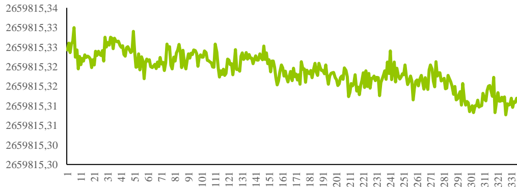
Figure 8. Expansion of the Y coordinate of the ANKARA station into time series
