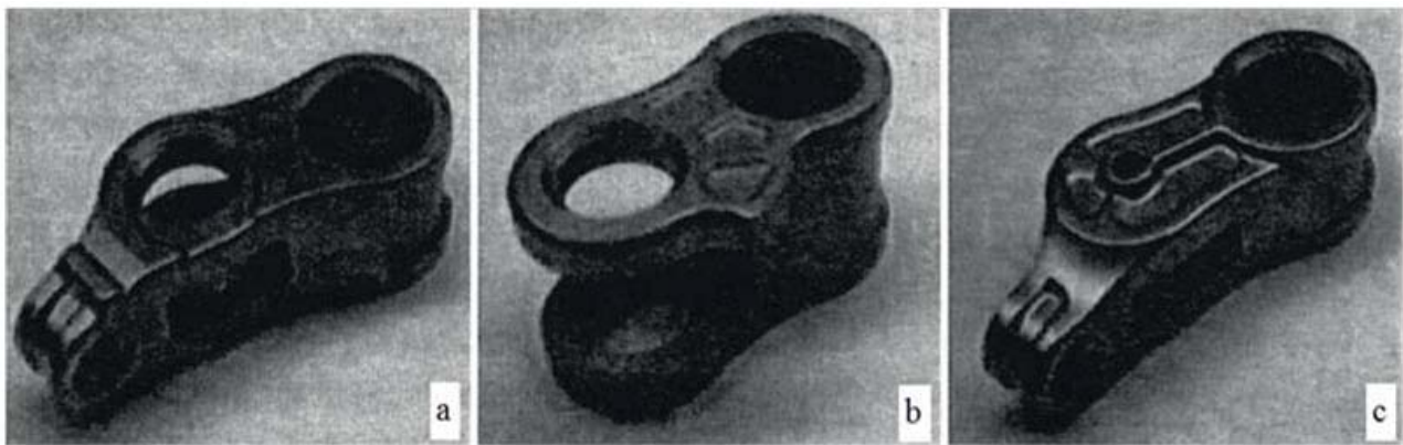
Figure 16. The swing arms manufactured by MIM for VTEC motor (HONDA): a) primary, b) middle c) secondary
