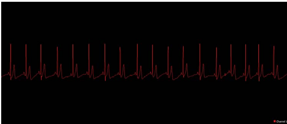
Figure 6: Wireless ECG measurement for distance of 20 meters.
