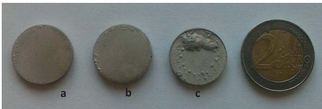
Figure 3: a) 550°C b) 600°C c) 610°C specimens sintered by induction.
