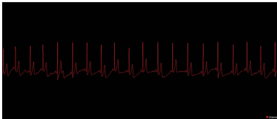
Figure 2: Wireless ECG measurement for distance of 5 meters.
