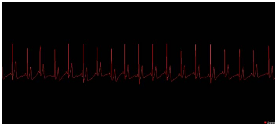
Figure 4: Wireless ECG measurement for distance of 10 meters.
