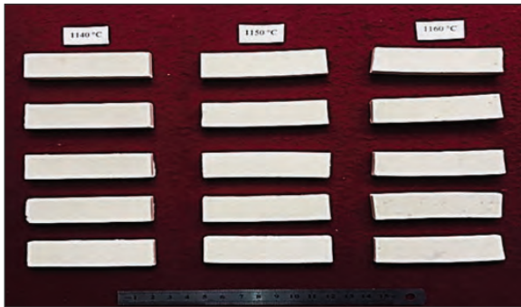
Figure 1- View of the materials fired (heated) at 1140, 1150 and 1160°C temperatures.
