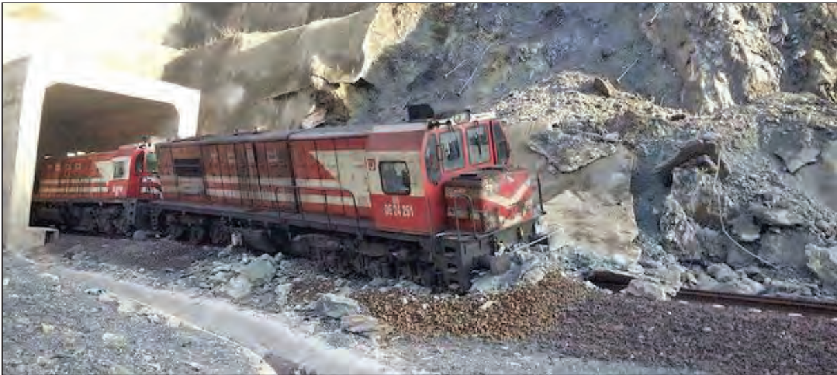
Figure 2- The landslide that occurred on 19 March 2017 at the exit of the tunnel on the new railway between Genç Beyhan and Süveran Locality, which had been built after Beyhan Dam, caused the locomotive to come out of the way ( http://www.hurriyet.com.tr/heyelan-nedeniyle-yuk-treni-raydan-çikti-40400338 19 Mart 2017).
