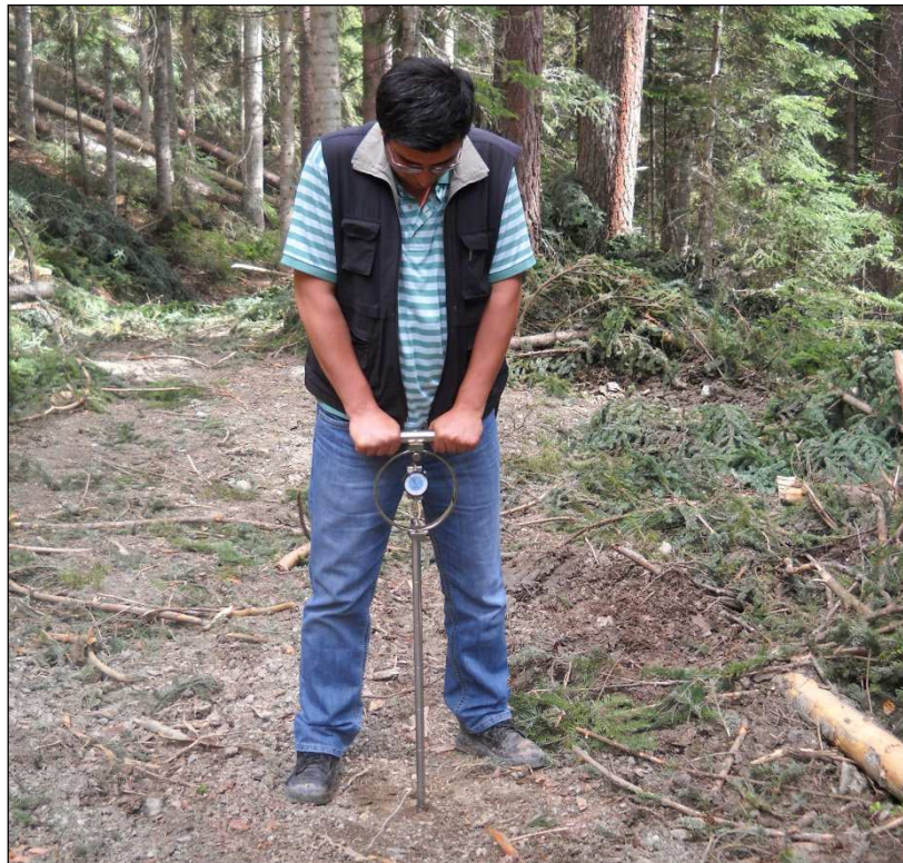
Figure 2. Hand-held cone (30°) penetrometer
