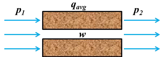
Figure 2. Fracture Core Seepage Diagram.
