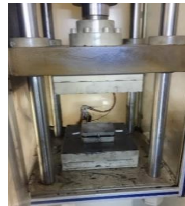
Figure 4. a) De-Mattia Specimen dimensions (ASTM D430-06) b) Mold c) Hot Press
