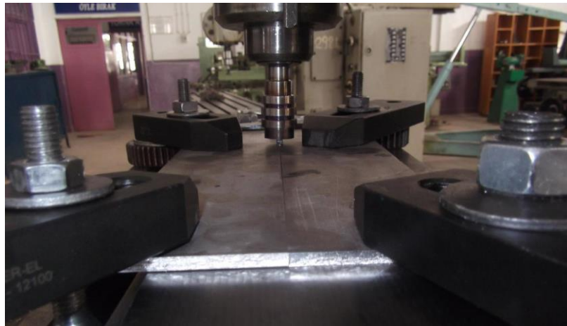
Figure 3. Fixture mechanism of the material couple to the milling machine
