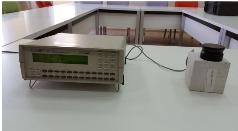
Fig. 3. The thermal property measurement device used in this study.
