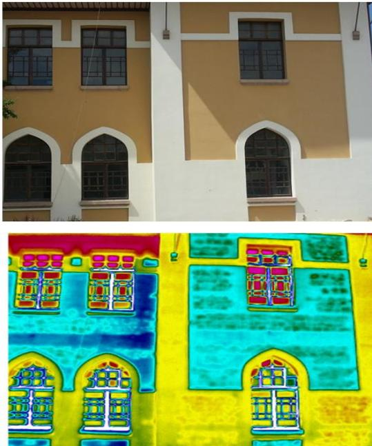
When the building materials were heated with heaters, the differences between the materials in the
