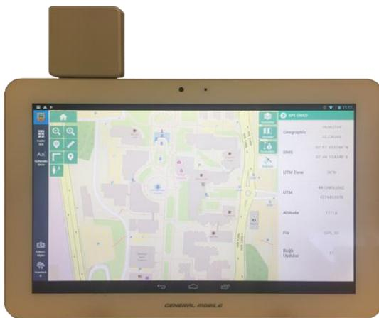
Figure 6. Tablet PC and external GNSS receiver
