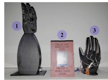
Fig. 1 Wireless hand rehabilitation system. (1) robot hand unit, (2) control center unit, (3) data glove unit
