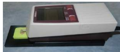
Figure 2. Representation of surface roughness evaluation with the tactile profilometer
