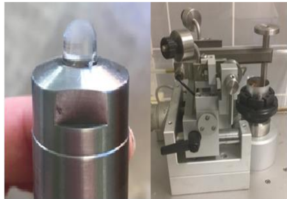
Figure 2. Modified tribometer probe with PDMS pin (on the left) and the CSM tribometer during experiments (on the right).
