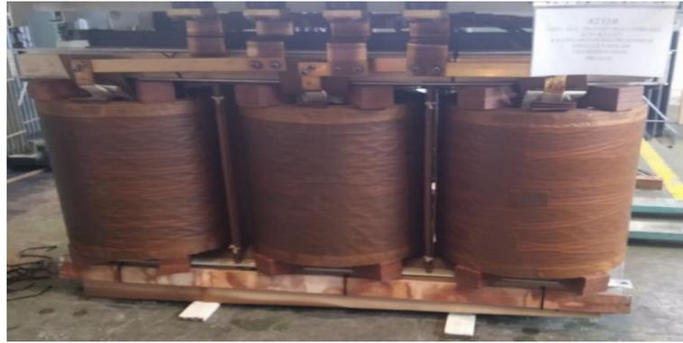
**Figure 3.1:** 34.5/4 kv 1250 kVA tested Transformer
