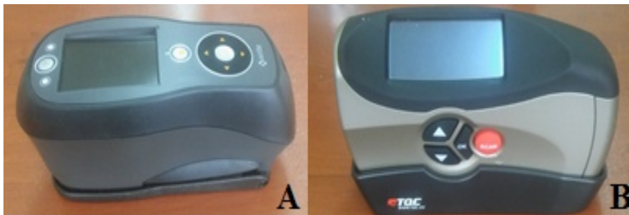
Figure 2. The colour measuring device (X-rite Ci62) (A) and the gloss meter (TQC PolyGloss GL0030) (B)
