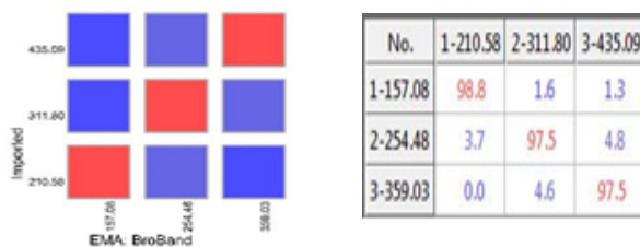
Figure 14. Determination of MAC for 10 mm-20 mm PUF reinforced sandwich beam
