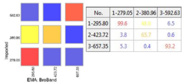
Figure 17. Determination of MAC for 40 mm-50 mm PUF reinforced sandwich beam
