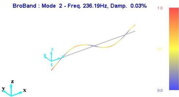
Figure 7. Second bending mode shape
