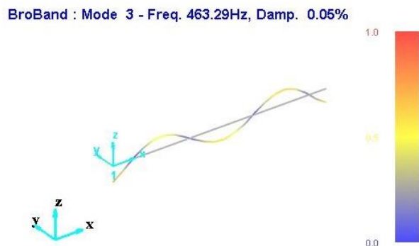
Figure 8. Third bending mode shape
