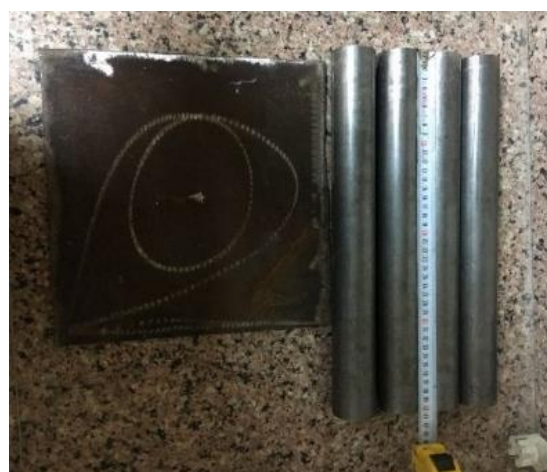
Figure2. Model Piles and Raft Foundation
