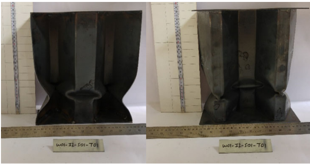
Figure 4. The impact deformation of the 2mm thick specimen
