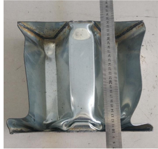
Figure 5. Drop test result for the 1.5mm thick specimen
