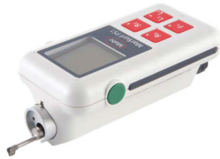
Figure 1. Desktop roughness measurement instrument
