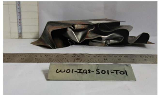
Figure 6. Drop test result for the 0.8mm thick specimen
