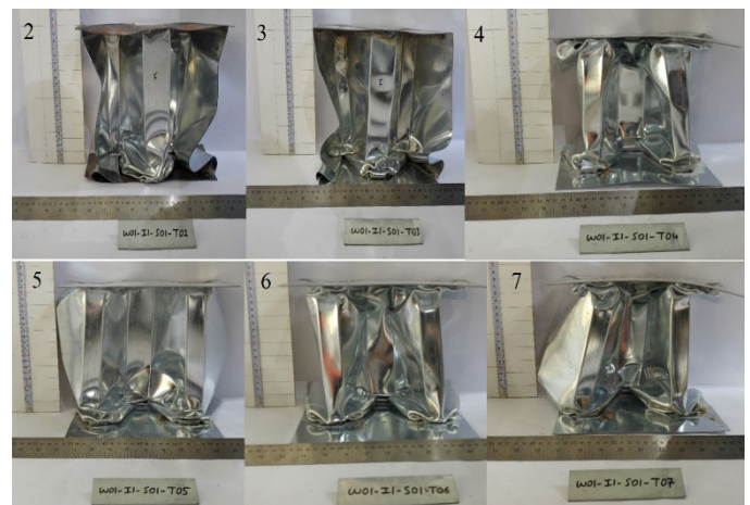
Figure 7. Drop test results of the 1mm thick specimen When the all experiments are considered, the results at Table 1 should be investigated.
