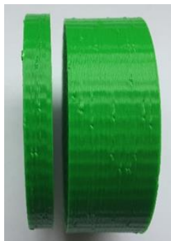
Figure 11. The objects printed with adaptive PID control at 100 mm/sec
