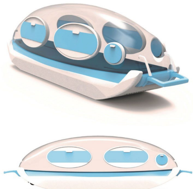
Figure 2- 3D design of the insulated patient transport capsule
