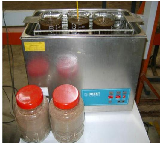
Fig 1. Crest Ultrasonics P1800D for PIAW derived zeolites optimization
