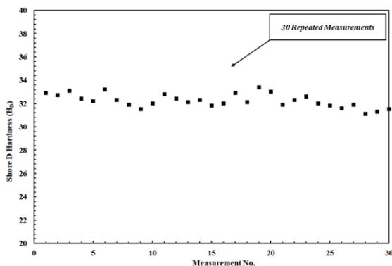
**Fig 3.** The overall shore D, (H<sub>D</sub>) hardness measurements on the material surface of PVC geomembrane samples
