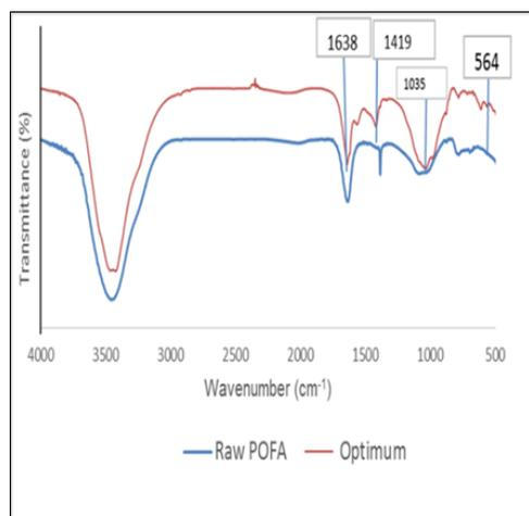
Fig 4. FTIR spectrum of POFA and zeolites (optimum)
