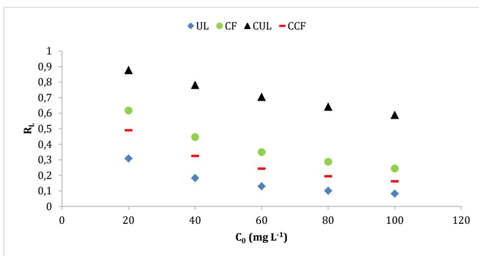
**Fig 3.** The equilibrium parameter (RL) of RBBR adsorption onto adsorbents
