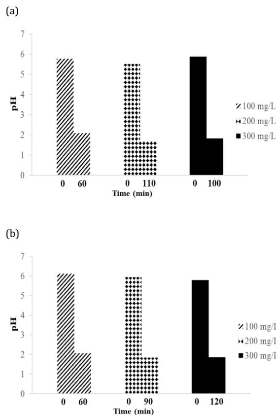
**Fig 4.** Changing pH at 25 °C with ozonation time for initial dye concentration:100, 200, 300 mg L<sup>-1</sup> (a) RB-5 and (b) RO-16
