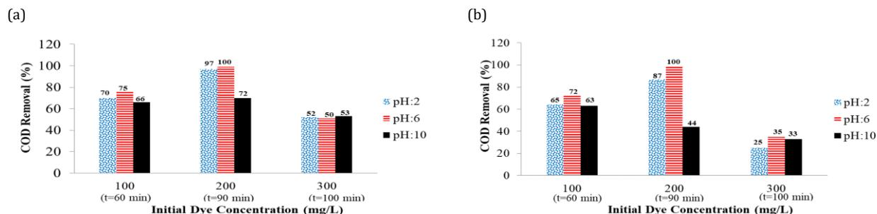
**Fig 5.** The efficiency of COD removal end of the ozonation for different initial dye concentration (100, 200, 300 mg L<sup>-1</sup>) and initial pH values (2, 6, 10) (a)RB-5 (b)RO-16
