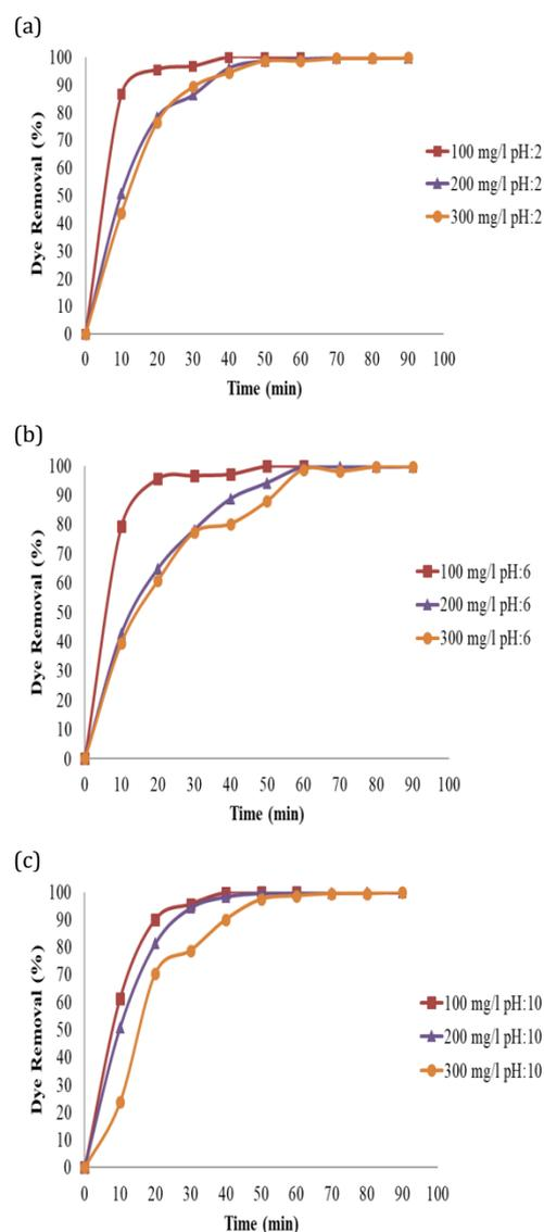
**Fig 2.** The changing of dye (RB-5) removal with ozonation time at different initial dye concentrations and pH ( $Q_{O_3}=5\text{g h}^{-1}$ ,  $T=25\pm 2^\circ\text{C}$ ) (a) pH:2; (b) pH:6; (c) pH:10
