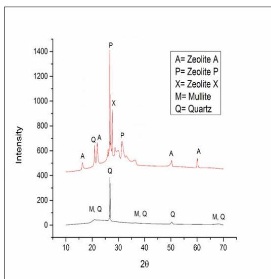
Fig 5. XRD diagram of POFA and zeolites (optimum)
