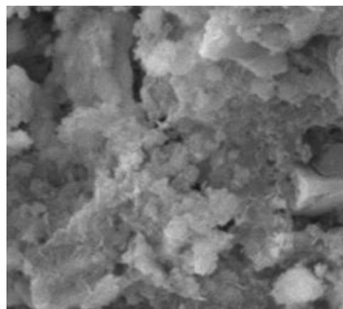
**Fig 3.** SEM images of zeolites at 1000 x magnification
