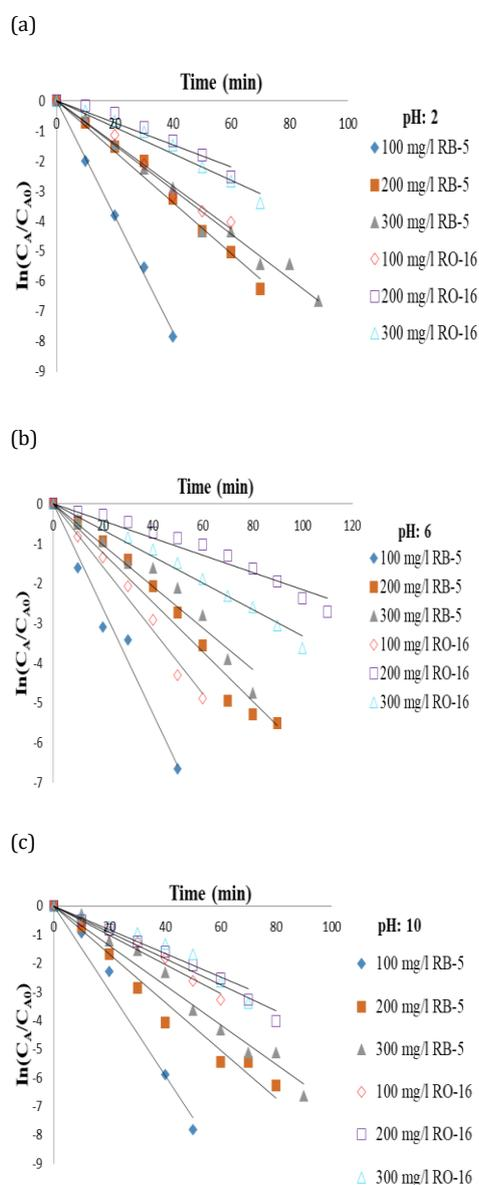
**Fig 6.** Linear transforms:  $\ln(C_A/C_{A0})$  versus time for decolorization of RB-5 and RO-16 during ozonation (a)pH:2 (b)pH:6 (c)pH:10 ( $Q_{O_3}=5 \text{ g h}^{-1}$ ,  $T=25\pm 2 \text{ }^\circ\text{C}$ )
