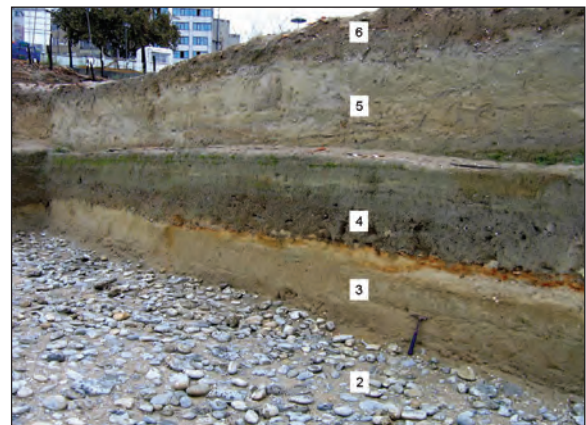
Figure 8- The relation of pebbly unit denoted as the Unit number 2, the 3 rd Unit represented by sand and the 4 th Unit which was deposited with a distinct contact is seen in photo. Oxidation around the bottom of the dark colored muddy 4 th unit is noticed. The 4 th unit is overlain by light colored 5 th Unit. The 6 th Unit is observed at the topmost.
