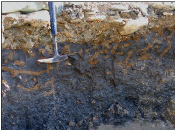
Figure 4- Relation of the 1 st Unit (dark gray colored marsh) and pebbly, sandy unit denoted as number 2. Nests of living organisms (burrows) are observed while the 2 nd unit deposits in the upper parts of the marsh. These burrows were filled by sand and fragmented shells.
