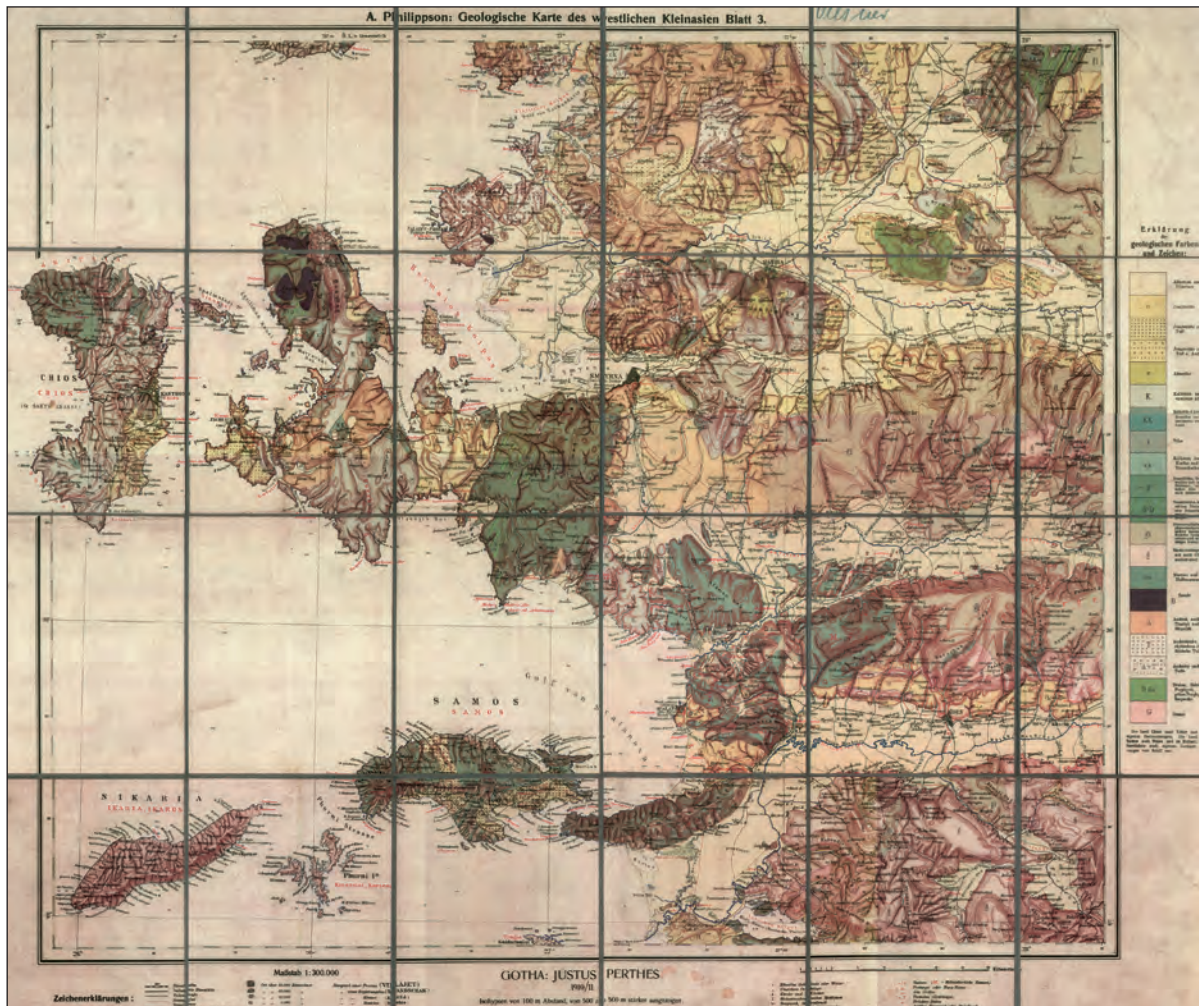
Figure 2- Geological map of the Western Anatolia (Philippon, 1911). Explanations: 1- Holocene and Pliocene, n2-Young Tertiary, 3- Tuff bearing Tertiary, 4- Tuff and andesite bearing Tertiary, e5-Lower Tertiary, k6- undated limestone, kk7-Cretaceous formation limestone (partly upper Jurassic), t8- Triassic, ck9-Carboniferous and Permo - Carboniferous calcereous, S10- clayey schist, diabase, greywacke, S+D11- clayey schist plenty of diabase and serpentine with veins, gl12- Mica schist and other crystalline schists (very little schistose gneiss), 913- Gneiss (very few micaschist), m14- Marble and semi-marble, B15-Basalt, A16- Andesite, trachyte and rhyolite, T17-Andesitic, trachytic and rhyolitic tuff, AYT18- Andesite and tuff, D,Se19- Diabase, gabbro, porphyrite, green porphyry serpentine, G20-Granite
