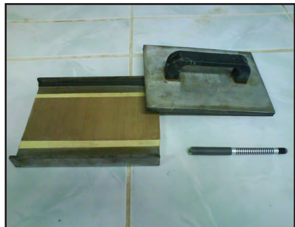
Figure 1- The rolling-device used to determine the plastic limit of soil samples.
