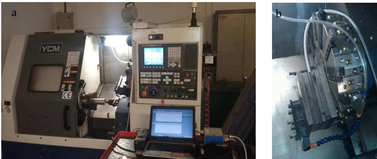
Figure 1. a) YCM GT-200A CNC lathe b) display of the dynamometer and cutting tool connected to the CNC machine
