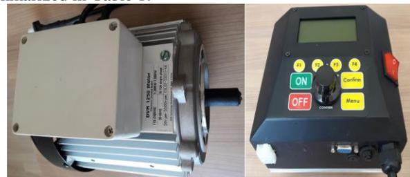
Fig. 5. SRM and controller unit
