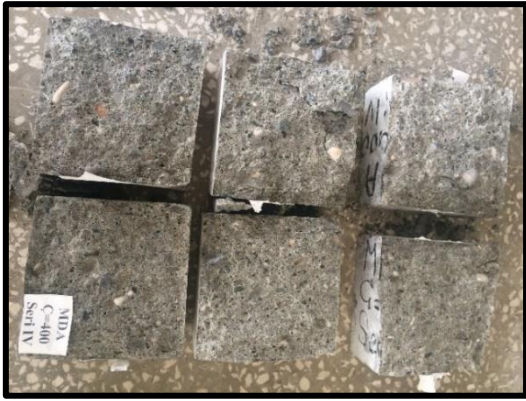
Figure 7. Broken sample surfaces
