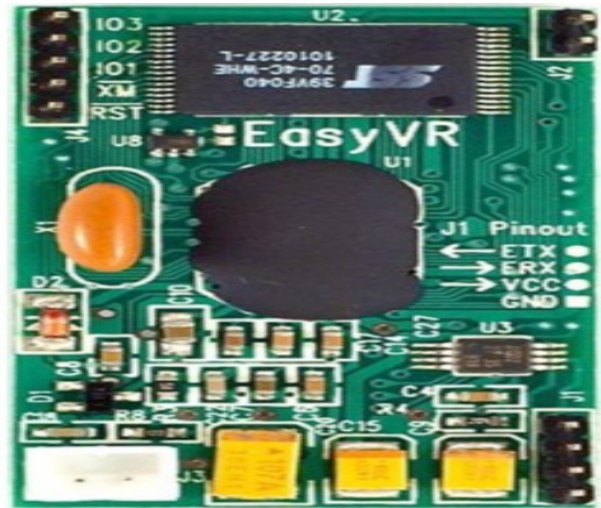
Figure 4. EasyVr voice-recognition module.
