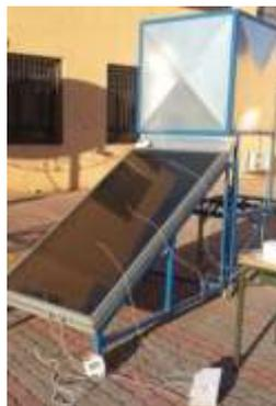
Figure 1. Photo of an indirect hybrid solar-electrical dryer.
